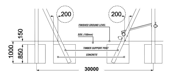
**ZW1-V2 / V3 TIMBERS** ARE SET an ANGLE - the 'edge' of the 800mm foundation measurement is 200mm away from the post where it 'MEETS' the ground level (CIRCLED ABOVE)
