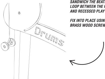
SANDWICH THE BEATER STEEL CORD LOOP BETWEEN THE PLAYTEC RING AND RECESSED PLAYTEC CIRCLE
