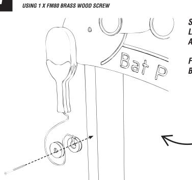
SANDWICH THE BEATER STEEL CORD LOOP BETWEEN THE PLAYTEC RING AND RECESSED PLAYTEC CIRCLE
