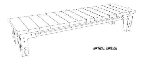
IMPORTANT - If foundation are required support legs will be have been extended 450mm
