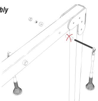
\*Ensure the nylocs are covered using end caps
