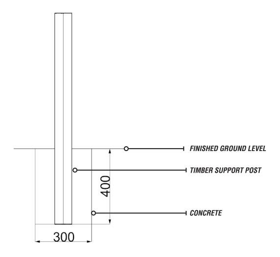
**1 SET TIMBER PLANTER INTO FOUNDATIONS** As shown on foundation details page
