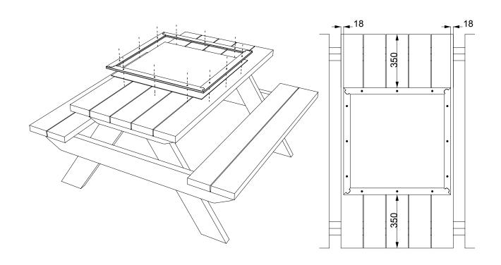
**TO INSTALL 2 BOARDS ON A 1.4M PICNIC TABLE, SCREW BOARD AND FRAME DOWN AS SHOWN BELOW** USING M6 X 40 SCREWS
