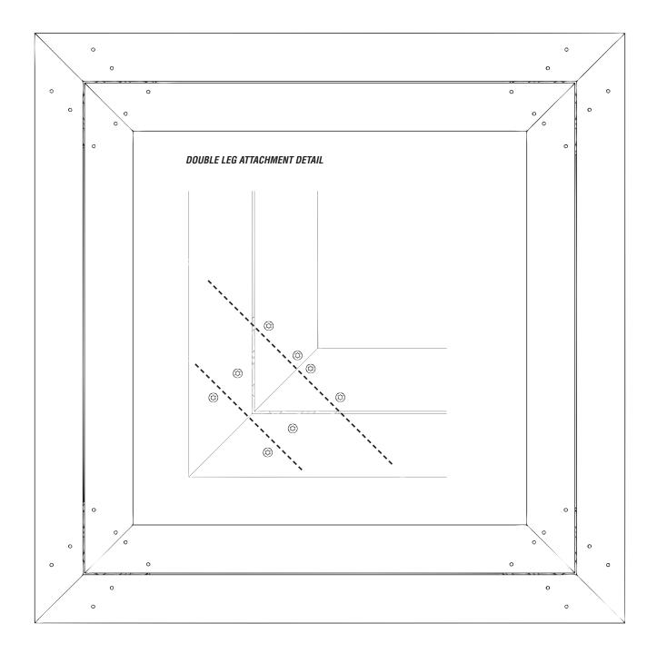
\*IMPOTANT - DASHED LINE SHOWS BOLT LOCATIONS FOR BENCH SUPPORTS - ensure the screws for the SLATS are postioned either side
